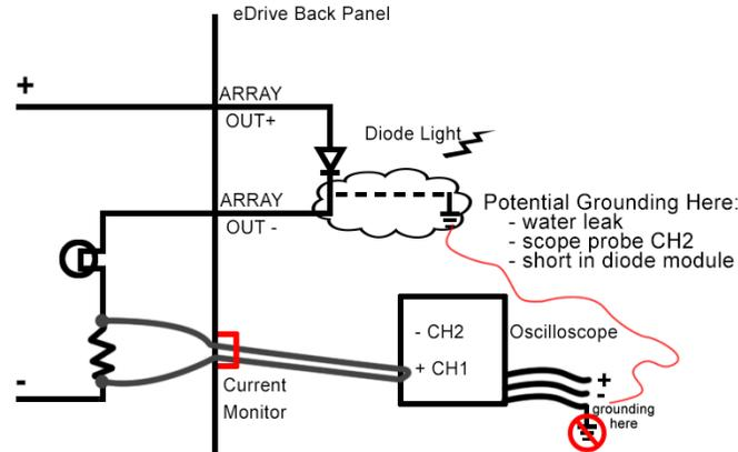
Figure B-2. Current Monitor Ground Loop
