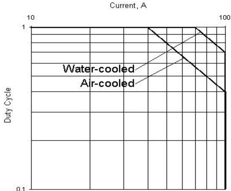
**Figure 2-7.** eDrive Configured at 100 A
