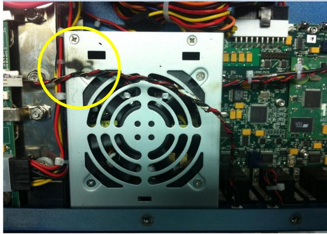
Figure 3-4. Burned Current Monitor Negative Wire
