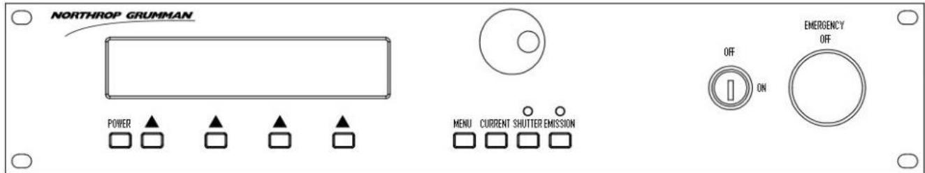
Figure 6-1. Front Panel Controls
