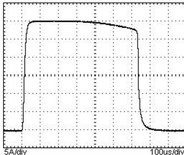
**Figure 3-6.** Waveform Characteristic for Long Current Pulse
