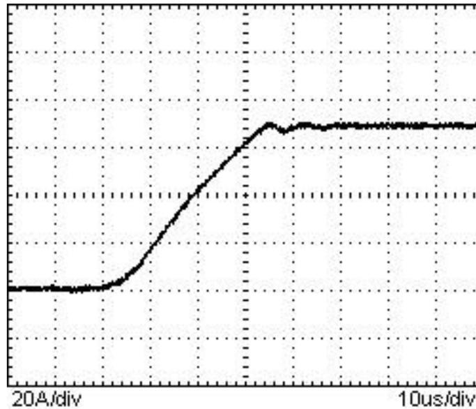
**Figure 3-7.** eDrive Set to Slew Rate Limit Control
