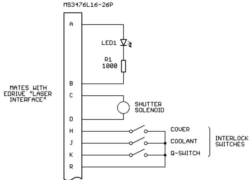
**Figure 4-2.** Laser Configuration for eDrive Nitro and Aero
