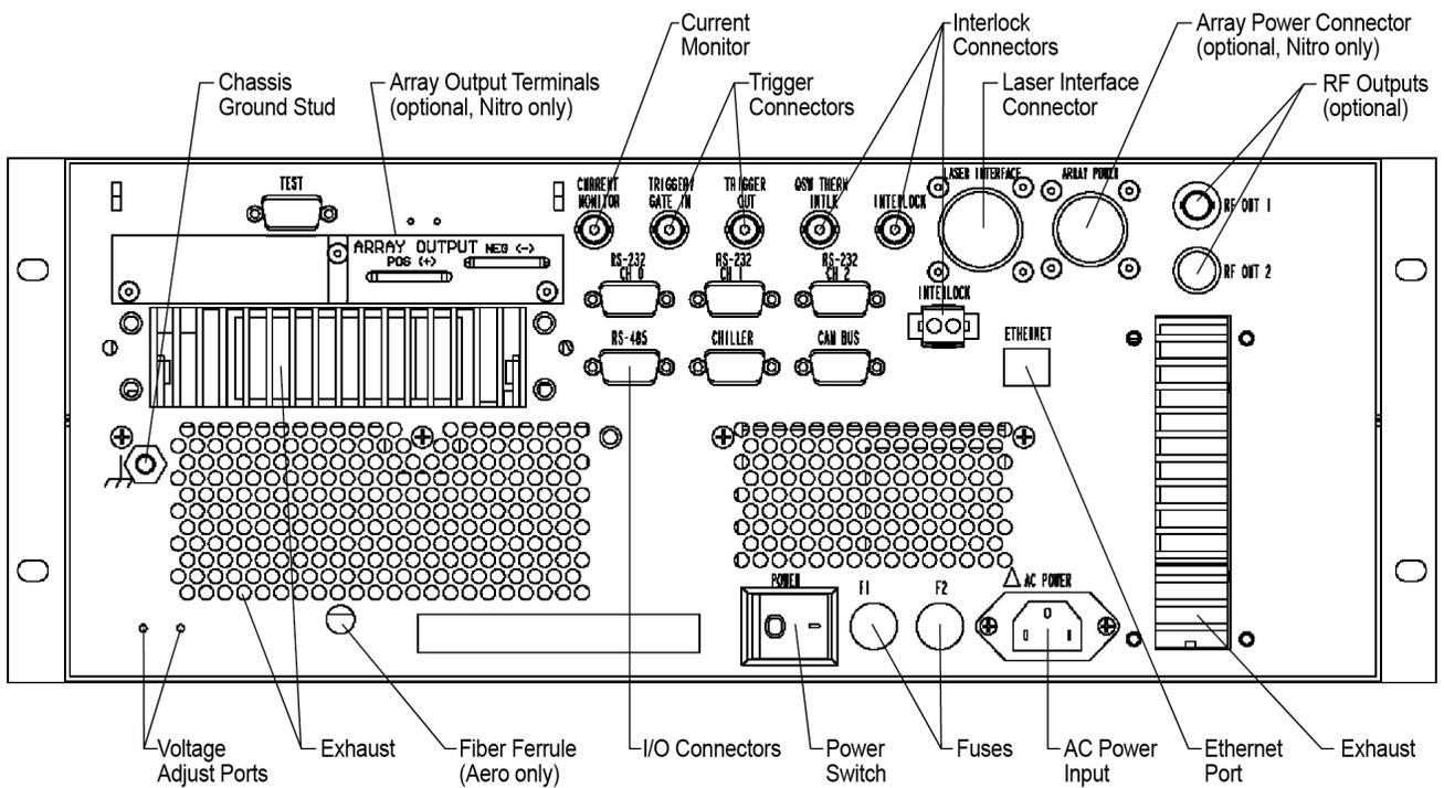
Figure 1-4. 4U eDrive Nitro and Aero Rear Panels
