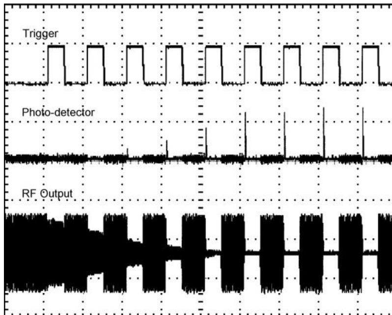
**Figure 3-11.** Typical Q-Switch Function
