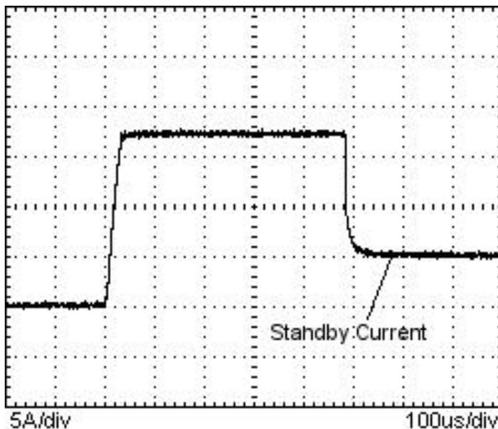
Figure 3-10. Standby Current Characteristics
