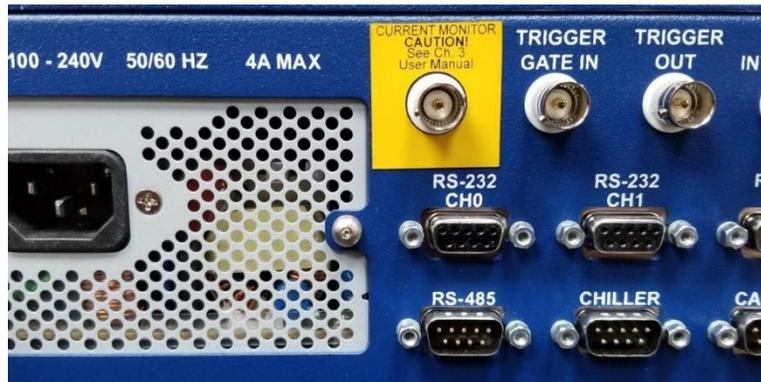
Figure B-1. Current Monitor Connector
