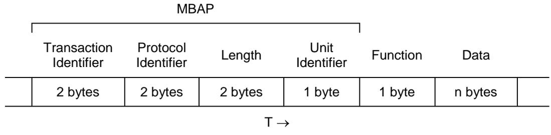
Figure 5-3. Message Frame for Ethernet Communications
