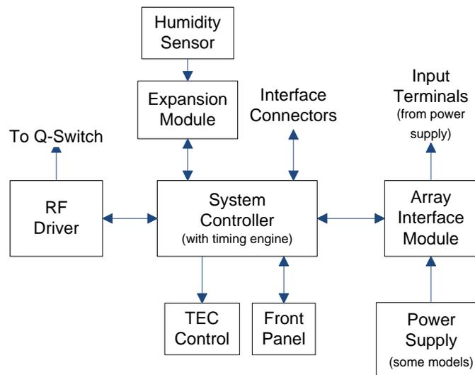
**Figure 2-2.** 4U eDrive Nitro Block Diagram
