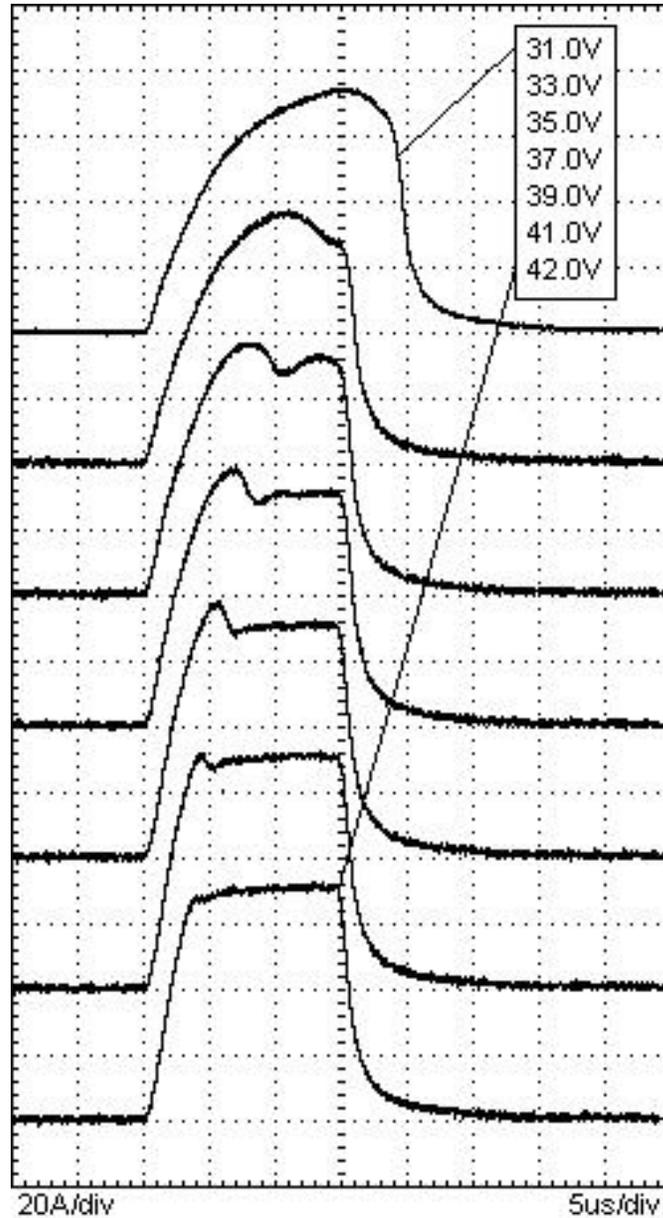
**Figure 3-9.** Waveform Characteristics with Varying Supply Voltages
