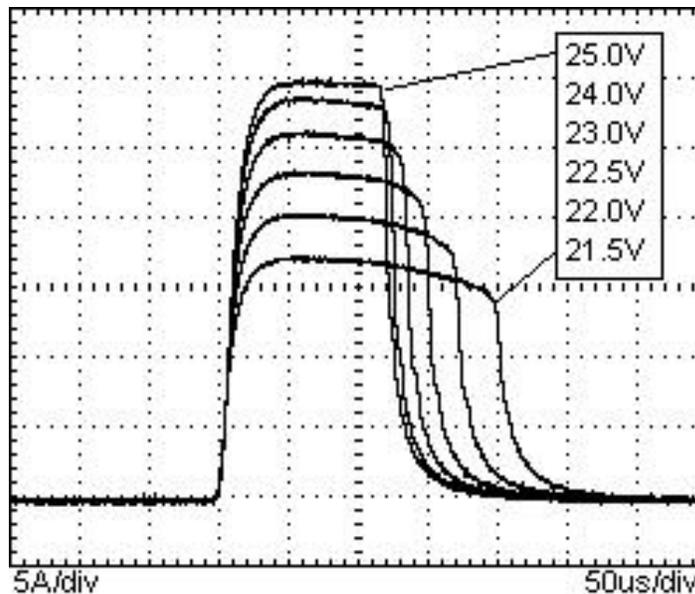
Figure 3-5. Waveform Characteristics for Power Supply Voltage Settings
