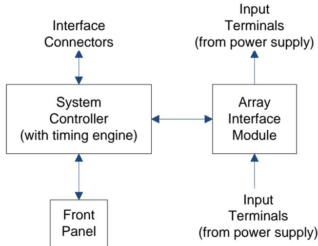
**Figure 2-1.** 2U eDrive Block Diagram
