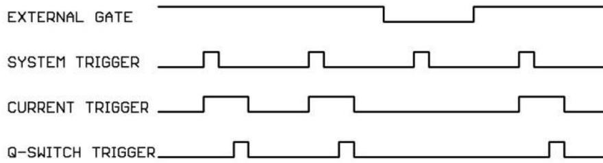
Figure 2-5. Timing for Internal Triggering with External Gating
