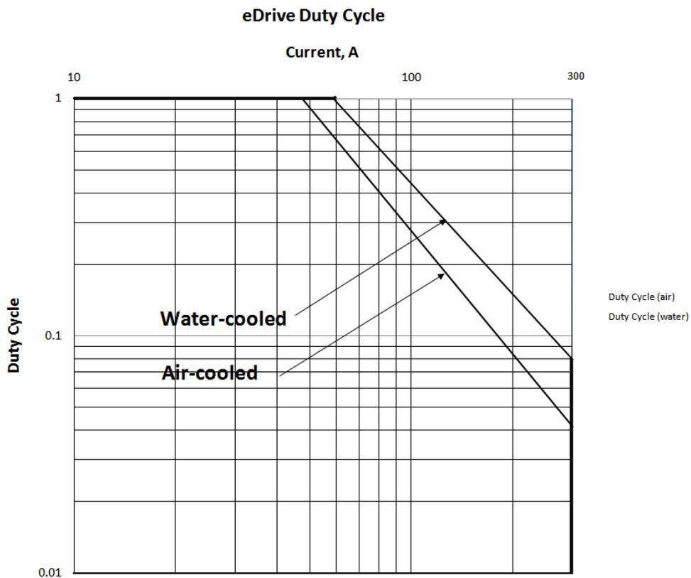
**Figure 2-8.** eDrive Configured at 300 A
