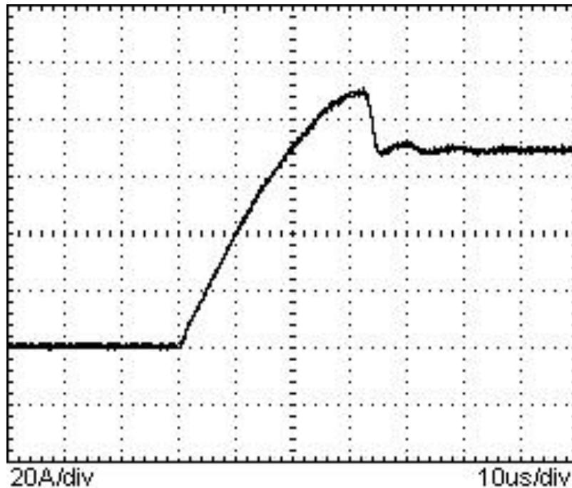
**Figure 3-7.** eDrive Not Set to Slew Rate Limit Control
