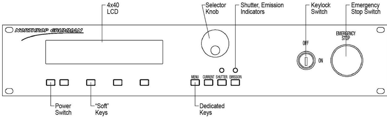
Figure 1-1. 2U eDrive Front Panel
