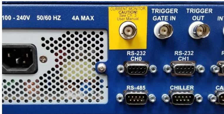
Figure 3-2. Current Monitor Connector
