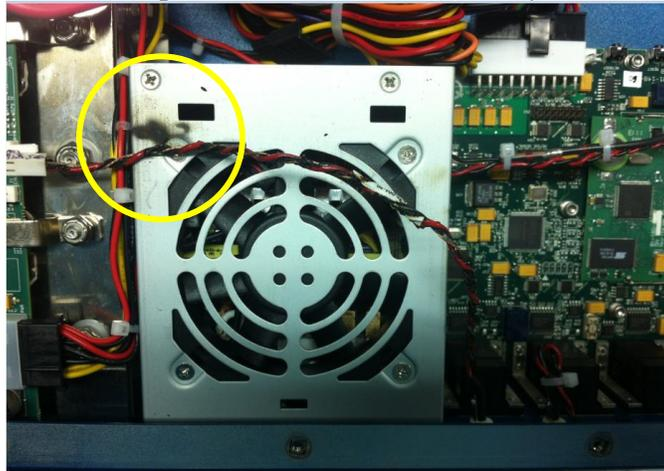
Figure B-3. Burned Current Monitor Negative Wire
