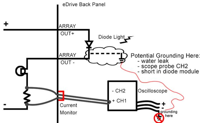
Figure 3-3. Current Monitor Ground Loop
